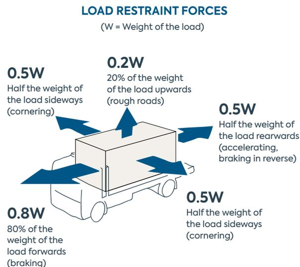
Note that these forces, and the forces that any load restraint system must be designed to meet or exceed, are equivalent to a low-speed collision between a heavy and light vehicle. That is, **any load restraint system for goods in/on a heavy vehicle or in a freight container must be capable of sustaining a low-speed collision between a heavy and light vehicle.**
